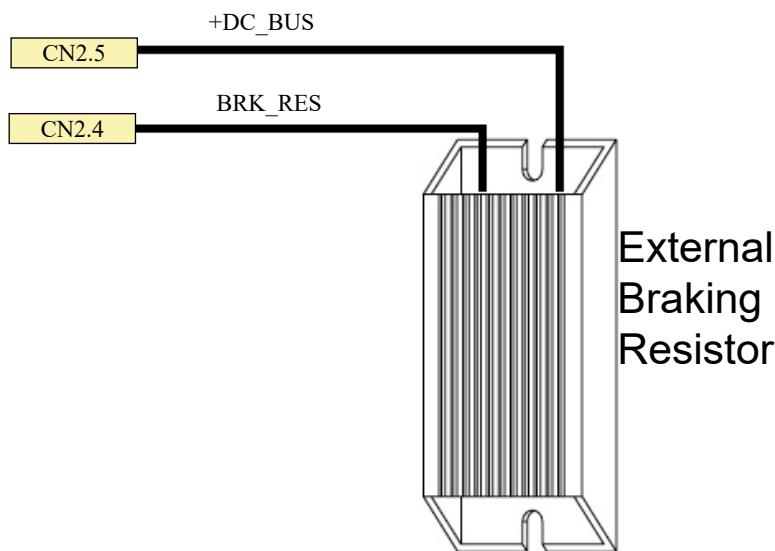
**!** *External braking resistor must be placed more than 50mm from the drive on nonflammable and heat resistant surfaces. The metal case of the braking resistor can reach high temperatures. Take all necessary measures to avoid possible contacts in the final installation.*
